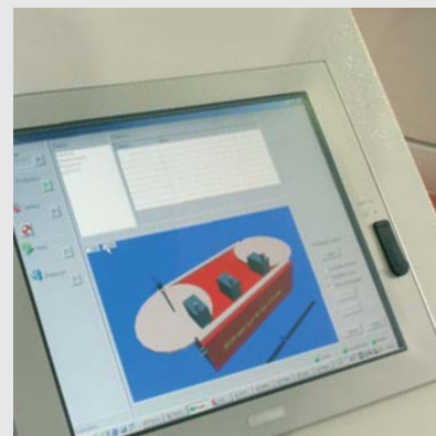
The HMI is designed to be operator friendly with advanced diagnostic and reporting capabilities via the touch screen.
