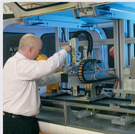
Unrivalled access is offered to operators for quick changeover and maintenance via the gull wing doors.
