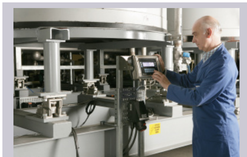
The design of the weight indicator means it can be operated directly in the hazardous area of this paint factory
