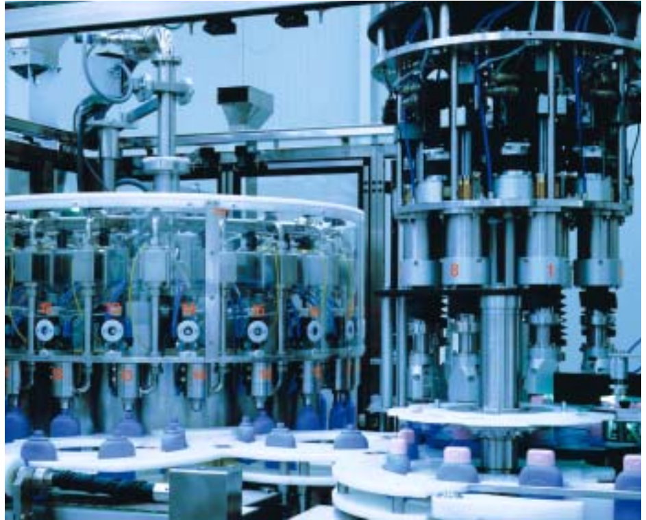
Servo drive: Ronchi has added servo cappers to its existing range of mechanically driven machines
