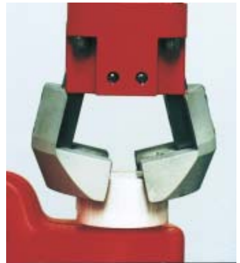
Torquing: Rubber lined fingers used by Cap Coder
