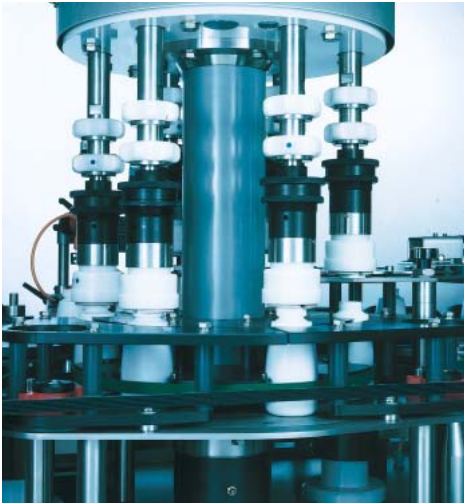
Cappers for Seven Seas: One of the two Dico 150-a-minute machines for cod liver oil tablet containers
