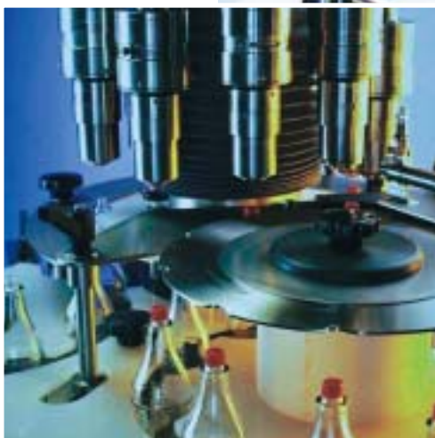
Standalone and combined: US Bottlers Machine Co has just developed a small frame filler-capper for pharmaceutical work (top), but also specialises in custom standalone cappers, such as this 14 head version (above)
