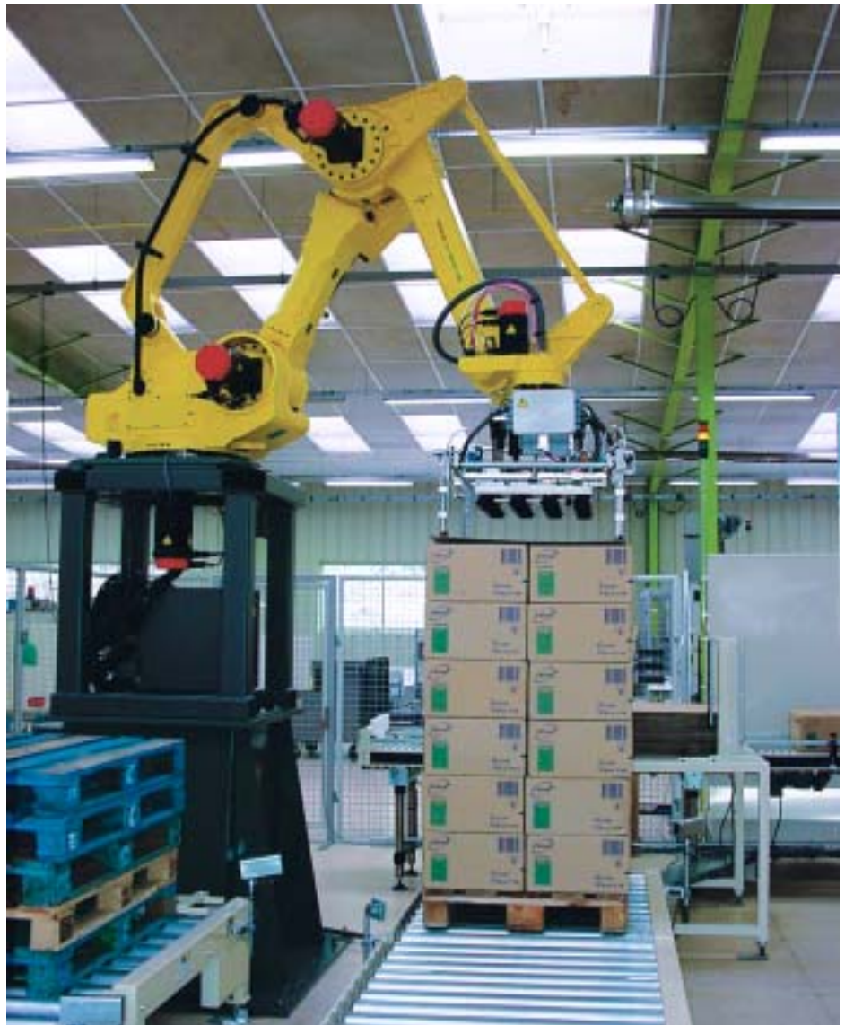
Handling almost anything: Cermex PR5 robotic palletiser uses the same head for a variety of products
