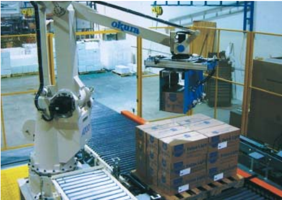
High weight capacity: The Okura A Series robot will handle a 200kg payload
