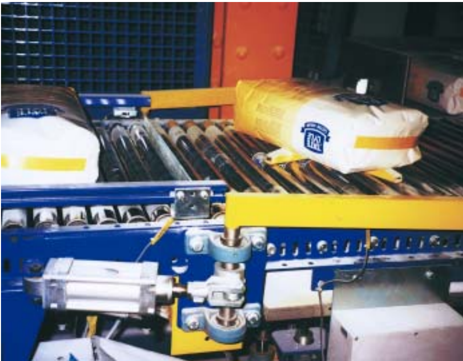
Turning unit: Dan Palletiser system for Tate & Lyle turns sack tops inwards to protect the handles
