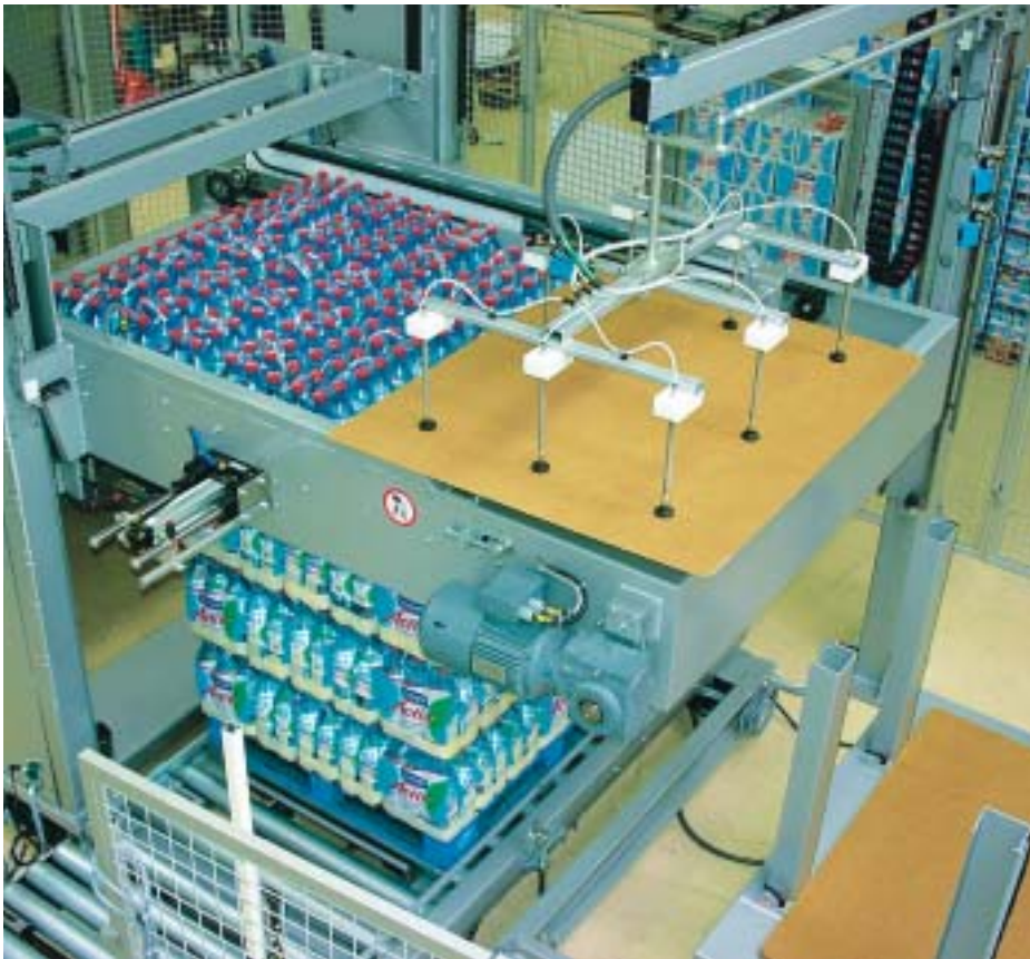
Recently redesigned: Cermex P4 palletiser can handle 60 cases or shrinkwrap packs a minute
