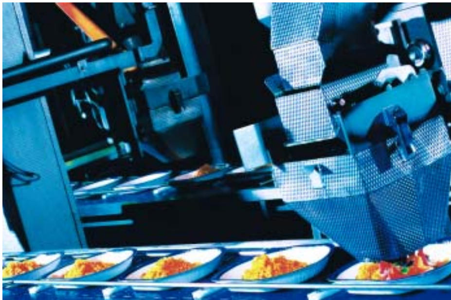
Automatic weighing: Ready meals components weighed out and deposited on a Bilwinco system
