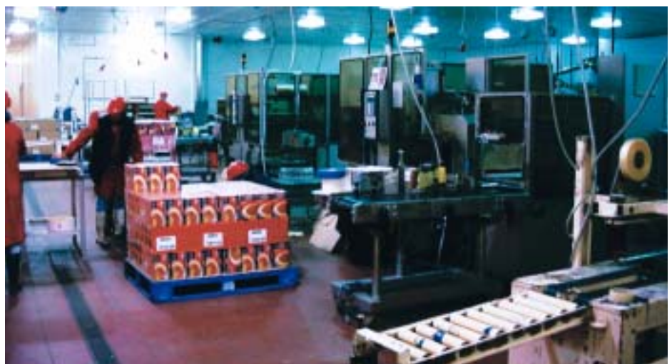
Final packaging: Finished frozen ready meals are stretchwrapped and palletised at Headland
