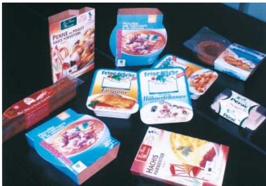
Board sleeving: A variety of trays can be sleeved by the Paker machine at speeds up to 300 a minute
