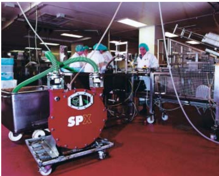
Peristaltic pumping: Watson-Marlow Bredel SPX40 handles onion gravy at Pork Farms Bowyers
