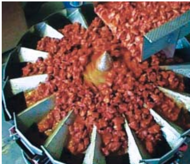
Vibratory feed: Multipond system is variable to handle difficult products
