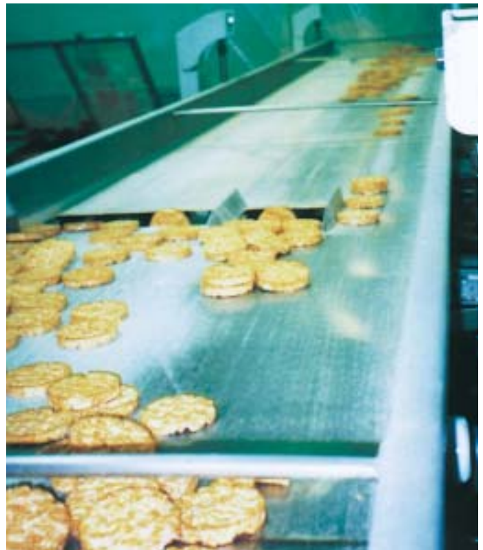
Gentle handling: Slipstick conveyor avoids risk of damage from vibration
