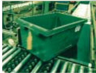
Sorting tote boxes: Tote boxes at JJB Sports distribution centre are marshalled and fed down a central conveyor (above) and then directed by sort modules (left) to spur lanes for individual shops
