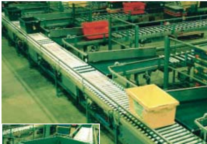
Sorting tote boxes: Tote boxes at JJB Sports distribution centre are marshalled and fed down a central conveyor (above) and then directed by sort modules (left) to spur lanes for individual shops
