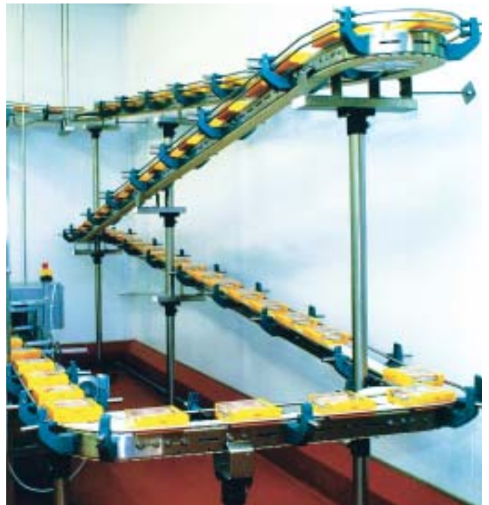
Saving space: FlexLink alpine conveyor at Laurens Patisseries
