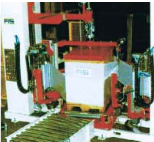
Twin film dispensers: FIS wrapper from Planet Flowline gives speeds up to 150 pallets an hour
