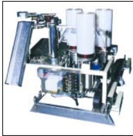
Automation: Above: the automatic film reel magazine for the Robopac high speed Genesis ring wrapper. Right: United Packaging automated this MR20 wrapper for bottlers Waters & Robson
