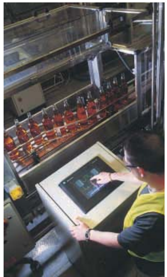
Intelligent control system: Machine performance data is available immediately to the operator
