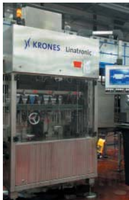
Empty bottle inspection: Linatronic multi-camera vision system checks for chips and other damage
