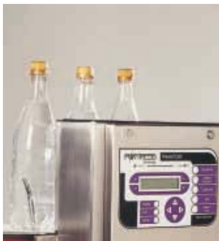
Looking for vent tubes: Metal detector from Fortress operates from the side of a conveyor
