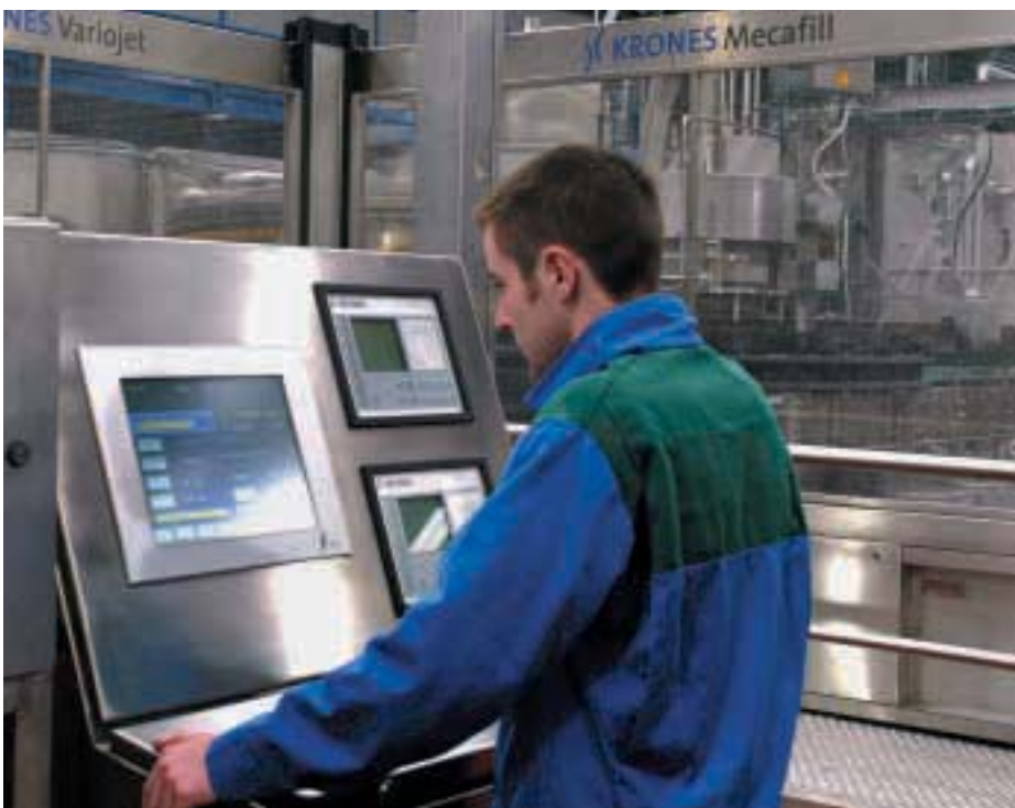
Line diagnostics: Terminal at the filler controls gathers data to give speeds, efficiencies and so forth
