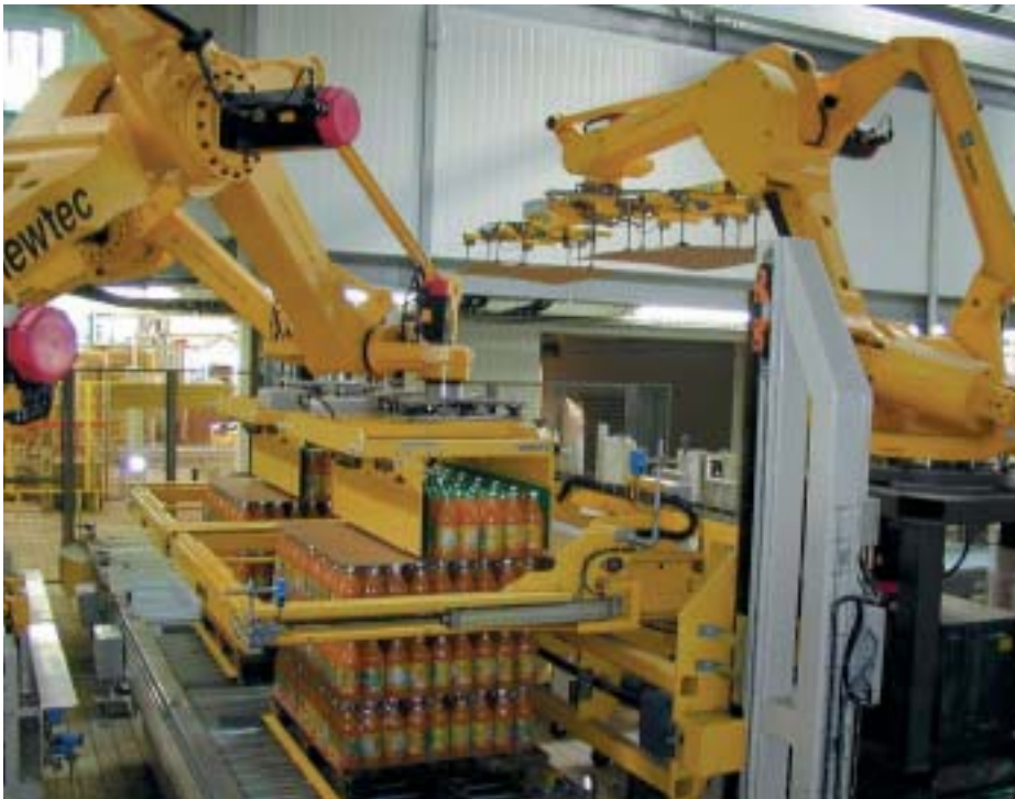
PET bottle handling in France: Robot palletisers installed by Newtec for Delifruits
