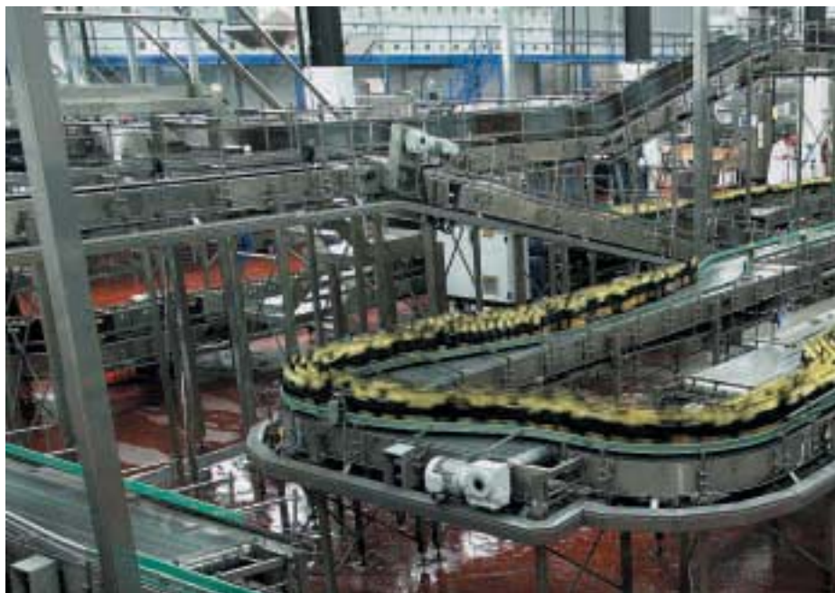
Eliminating foreign bottles: After decrating the Sekamat sorter (top right) checks bottle profile
