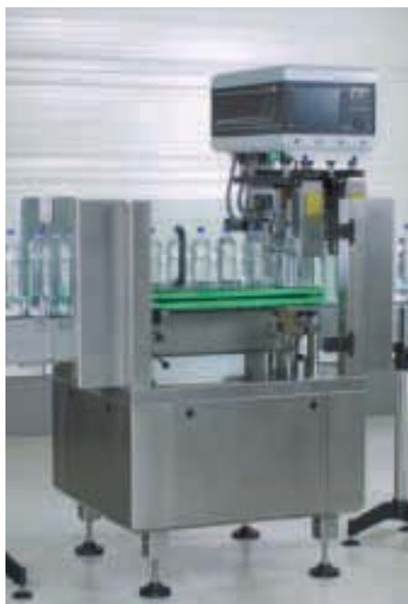
Checked by a squeeze: Pressure is applied to filled bottles by the new Heuft leak detector
