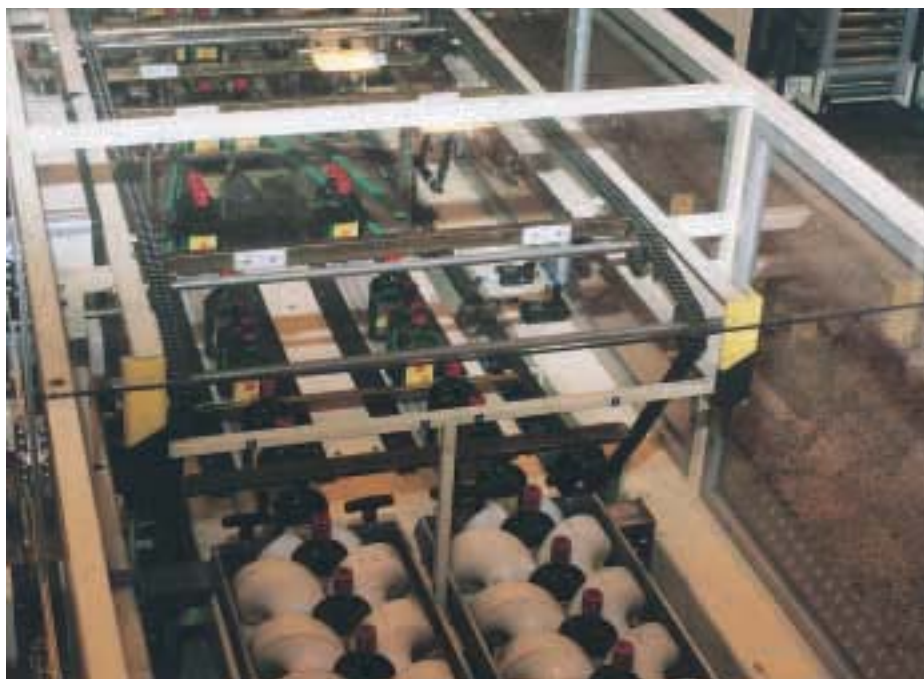
Continuous motion: Scroll infeed to Cermex TS tray packer and shrinkwrapping machine
