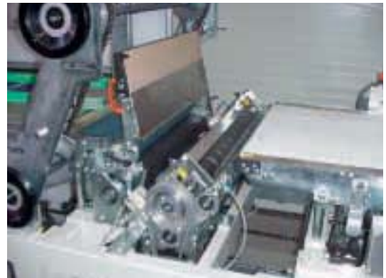
Film drive: Dimac's new system, shown open
