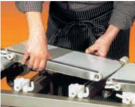
Easier cleaning: New drive system and belt layout eases cleaning on Bizerba's CWM system
