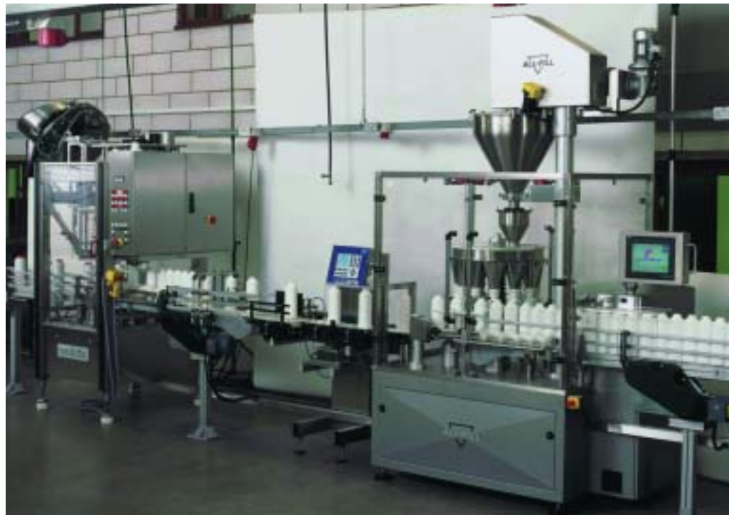
Talcum powder line: All-Fill turnkey installation is based on a rotary auger filler
