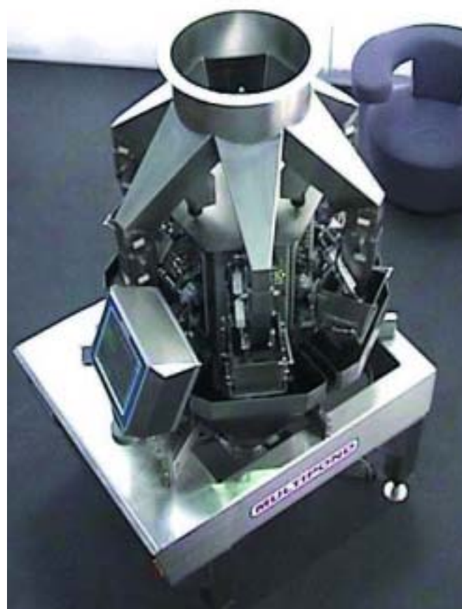
Multihed for powder: Multipond's new DW640A in six-head format
