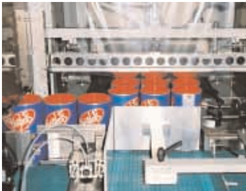
Above: Tray stacking station on the Polypack PH-24L shrinkwrapper Left: Jacobs has installed a YPS shrink-wrapping line for Twiglets tins
