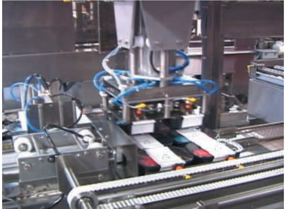
Above: Tray stacking station on the Polypack PH-24L shrinkwrapper Left: Jacobs has installed a YPS shrink-wrapping line for Twiglets tins
