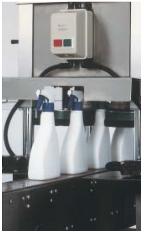
No change parts: Newman's cap tightener for trigger sprays and pumps adjusts to different sizes
