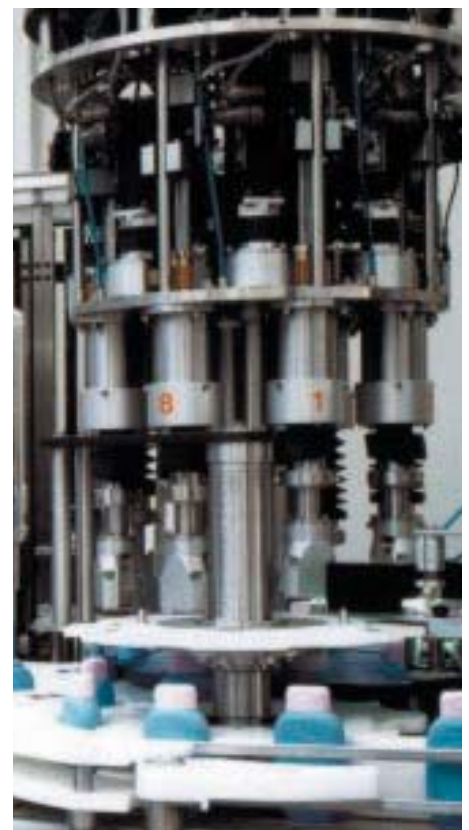
Fewer mechanical parts: Ronchi servo driven rotary cappers give speeds up to 300 a minute
