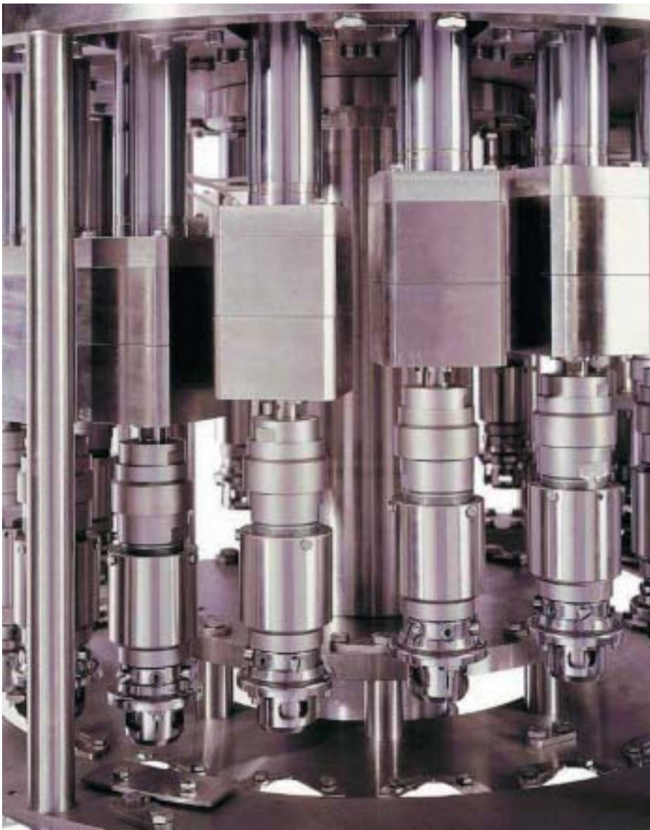
Individual drive: Zalkin cappers can be supplied with brushless motors on each capping head
