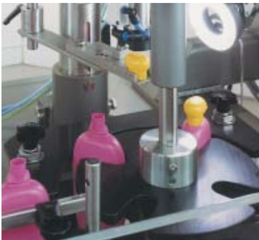
Servo capper: Dico 100S can be equipped with a colour vision system
