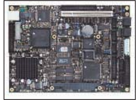
Single board: Arcom's SBC-GX1 high performance fanless single board computer
