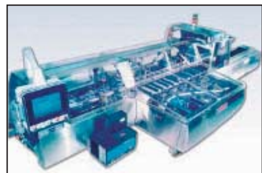
Soft control: Bradman-Lake SL9000 end-load cartoner is under softPLC control
