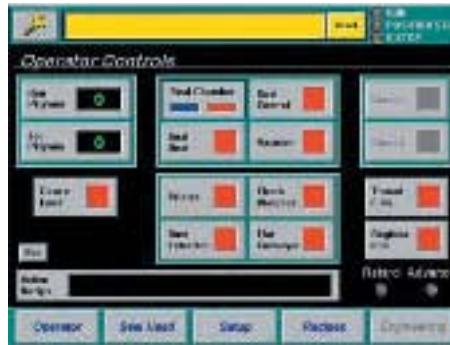
Combined system: Doyen Medipharm 4SS uses a PC display and PLC machine control
