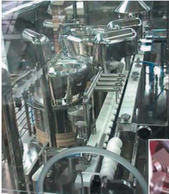
Filling injectables: Above: Compact MAR M53 filler for vials. Right: Pre-heat and ampoule sealing station on the Rota eight-head in-line filler
