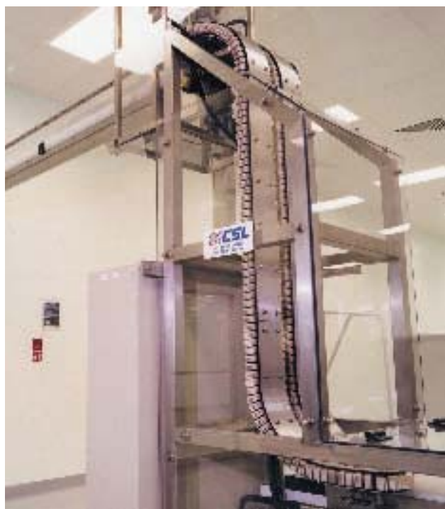
Up and over: Elevator section of the spray bottle conveyor
