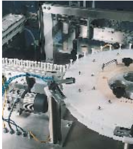
Syringe labeller: Newman VAL 550 showing the starwheel arrangement
