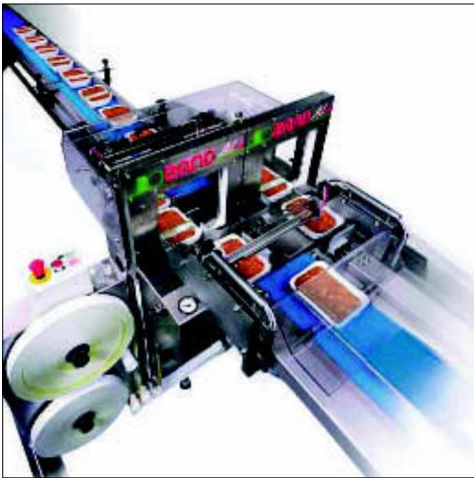
Labelling trays: Automatic BandAll machine offers alternative to sleeves
