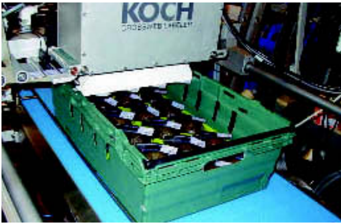
Reducing labour cost: Modified Koch labeller can handle avocados
