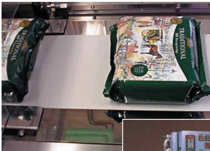
Bigger bags: Sachets of Ringtons tea are now collated and packed into outer bags on a Fuji system from Paramount
