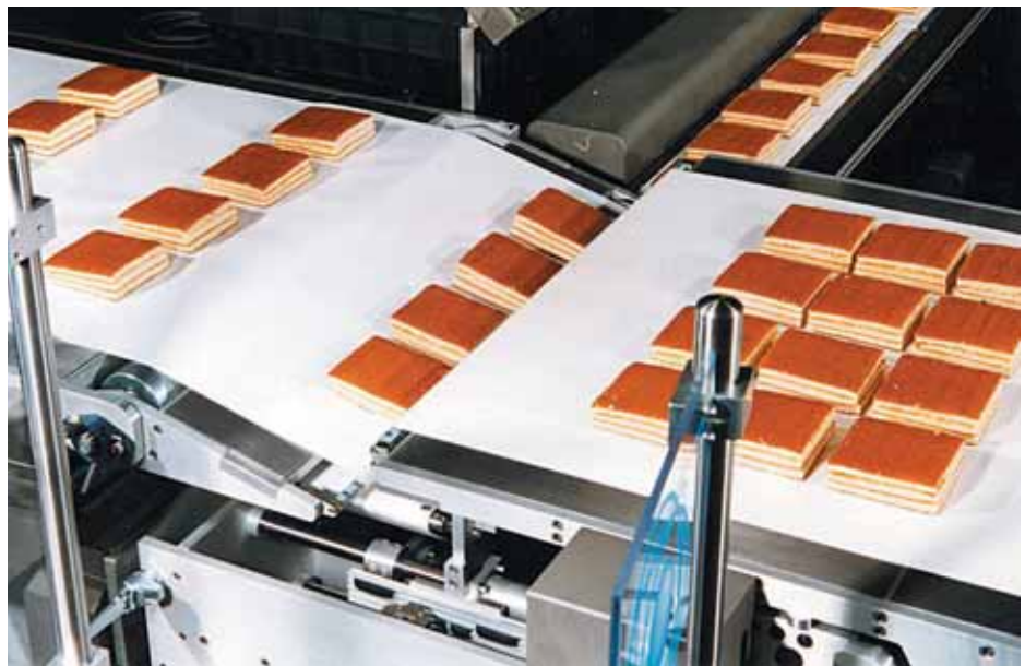
Feed system: Record Selecta transfers rows at 90 deg to the Flowfeed system of the wrapper
