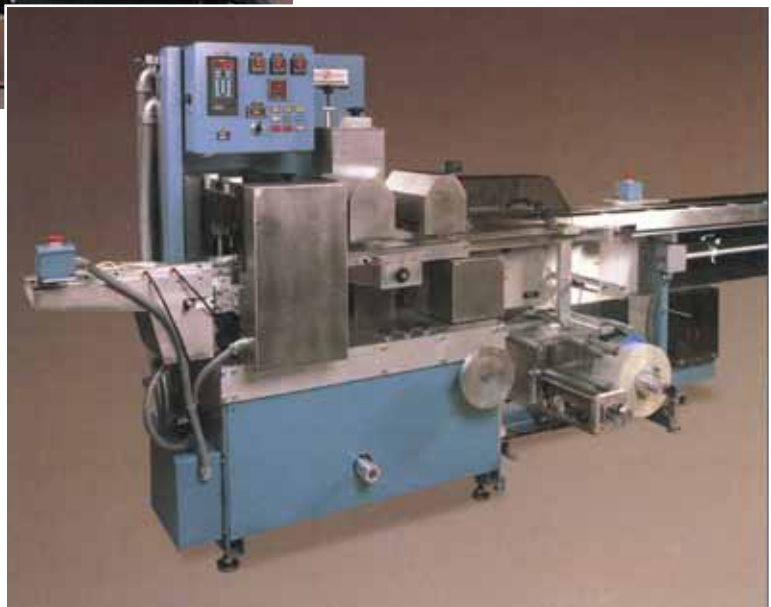
Dedicated wrapper: GPS-10 produces food service kits at 240 a minute
