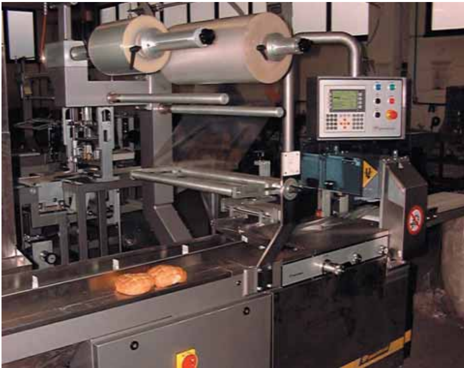
High speed: Adpak's new Gemini wrapper employs three separate motors
