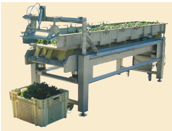
Cleaning by vibration: High amplitude system from Wright
