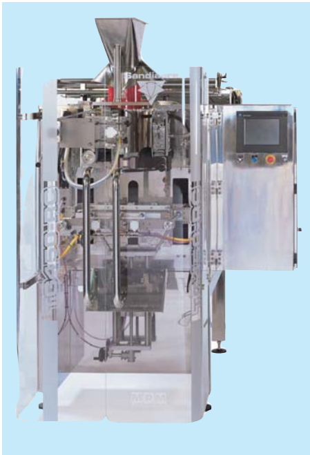
Big bags for potatoes: Sandiacre TG450-RC runs at speeds up to 120 a minute
