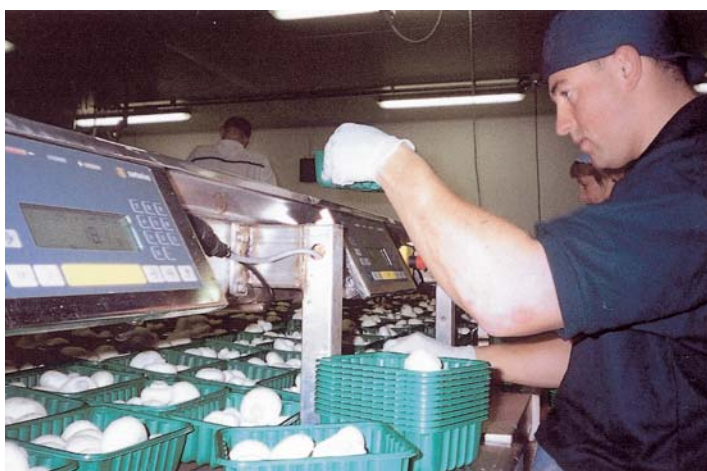
Reducing giveaway: J Rothwell has installed six SEB scales from Sartorius
