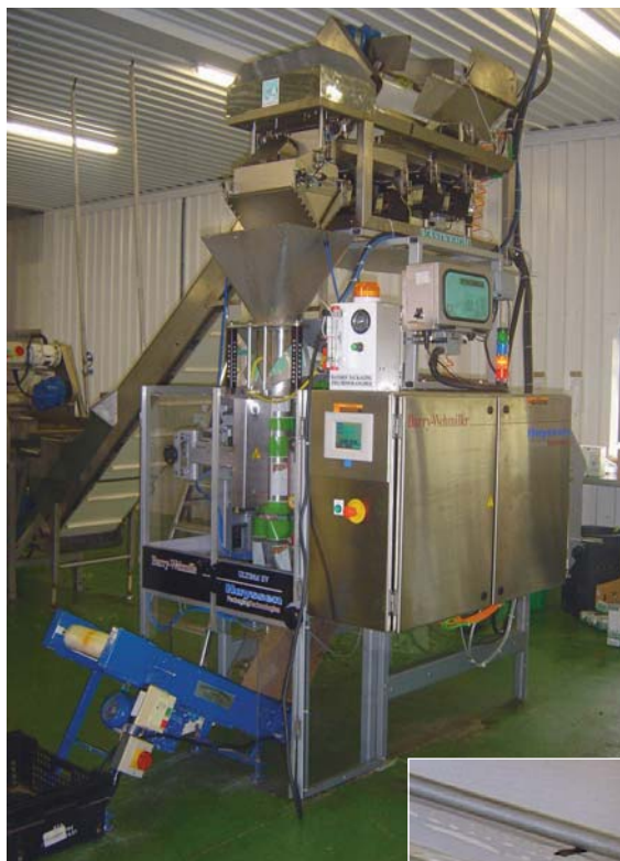
Reduced cost: Hayssen Ultima SV 'E' bagger - built with some recycled material - has allowed D Laurie & Sons, Norfolk, to move from pre-made bags to automatic form-fill-seal at reduced cost
