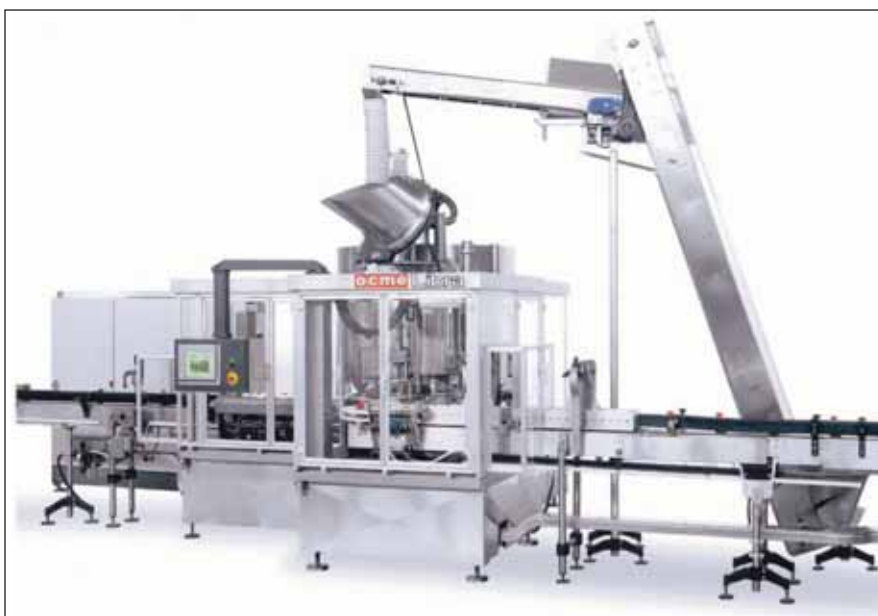
Fill by weight: Ocme Libra net weight filling machine and capper
