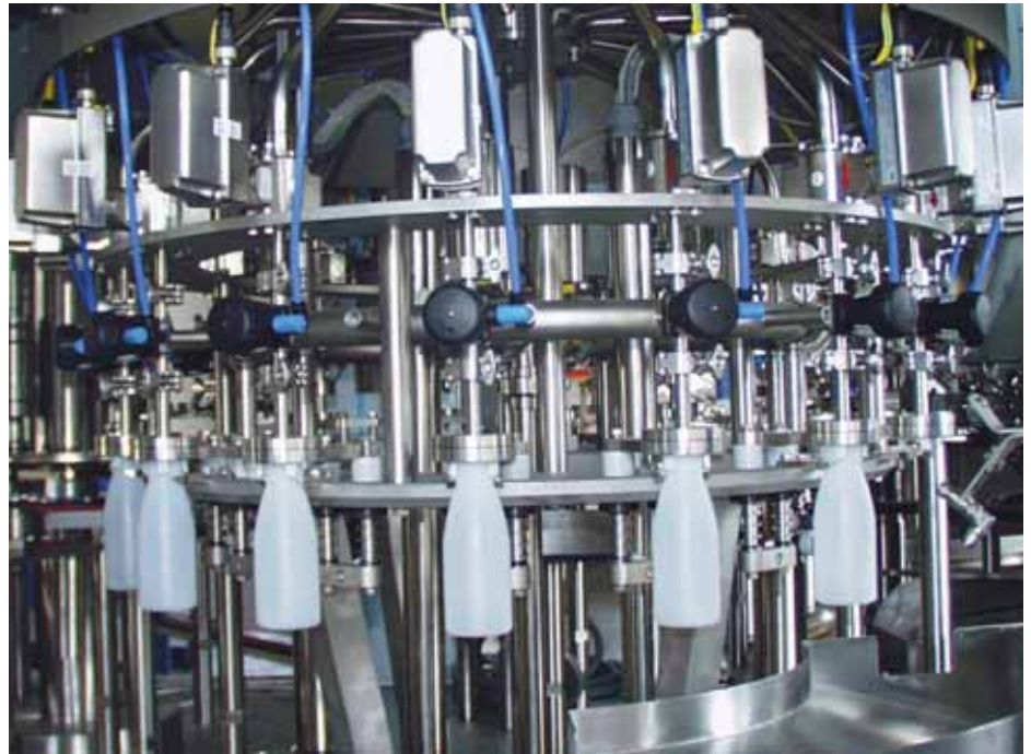
Flowmeter filler Berchi has launched its Unitronic machine for still drinks such as water and juices
