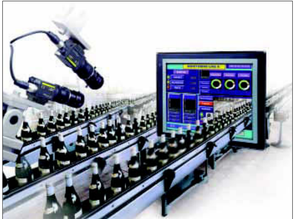
Quality control: A typical environment in which a vision system would be installed. Here it inspects characteristics of the bottle, which could include label placement, printed data on the label or checking that the closure is correctly fitted. (Picture: Omron Electronics)
