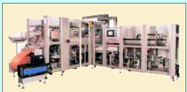
Wrapping for savings: Cartons are overwrapped in kraft paper by the Marden Edwards KPB 650
