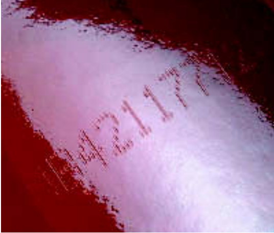
Hot marking: Dot matrix codes are applied to hot glass by the Linx Xymark BBH laser
