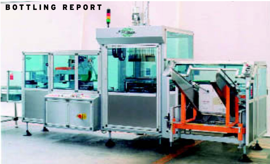
Top-loading monobloc: Mondo & Scaglione Impack machine from Sealed Air
