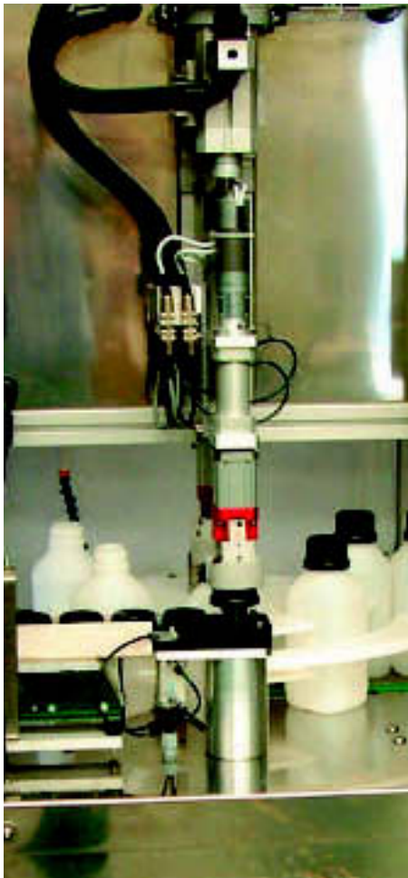
Versatile capper: Cap Coder's new CC560 machine
