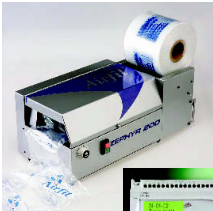
Mini controls: Above: Small machines such as this airbag maker are now frequently controlled by a tiny logic block. Right: Tiny PLCs or logic blocks have carved a niche for themselves in large machine control systems as well as standalone systems on smaller items of equipment
