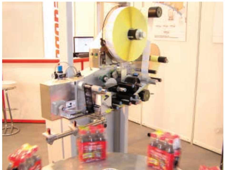
Non-contact: Logopak introduced the 906F front-of-pack print-apply labeller at Interpack
