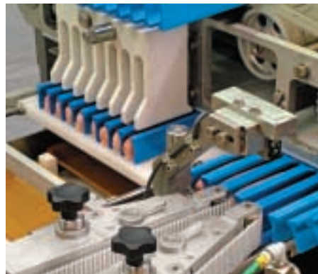
Collating machine: Individual sausages are accepted into pockets created by sets of fingers
