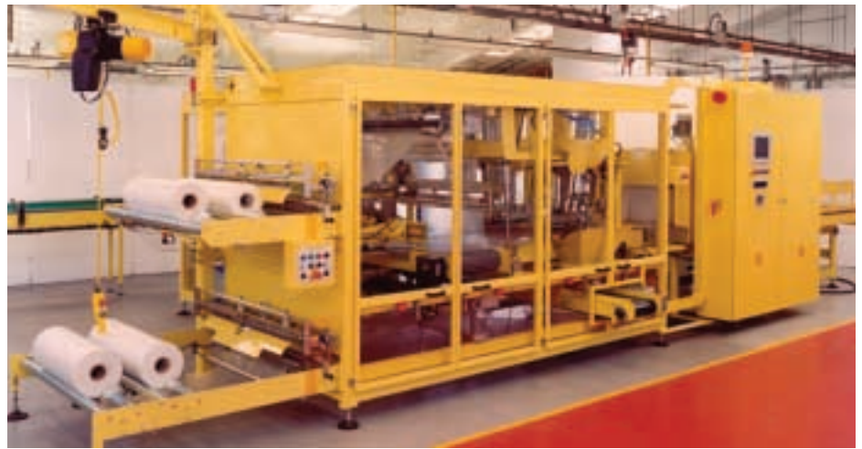
Faster and more flexible: Europack collator and shrink-wrapper equipped with servo drive
