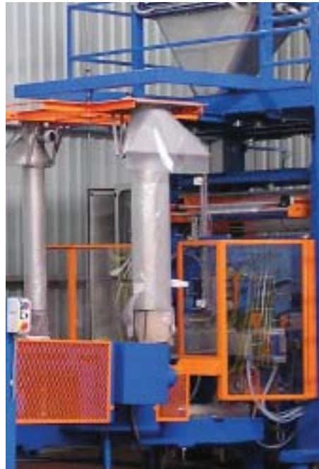
Fast changeover: CV2080 bagger at Peacock carries its large forming tubes on a carousel
