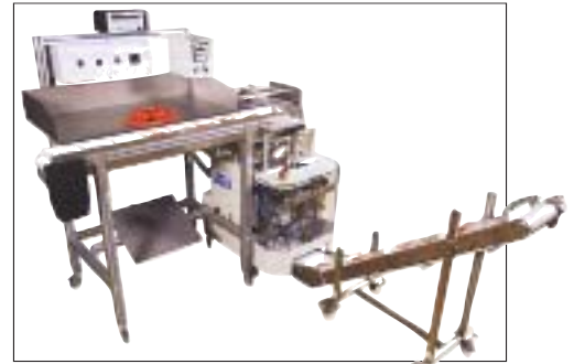
Packing module: Compact Audion 1901C bagger with sorting table and outfeed conveyor
