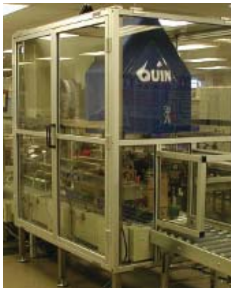
Motion control expertise: Quin Systems demonstrated this pick-and-place case-packer
