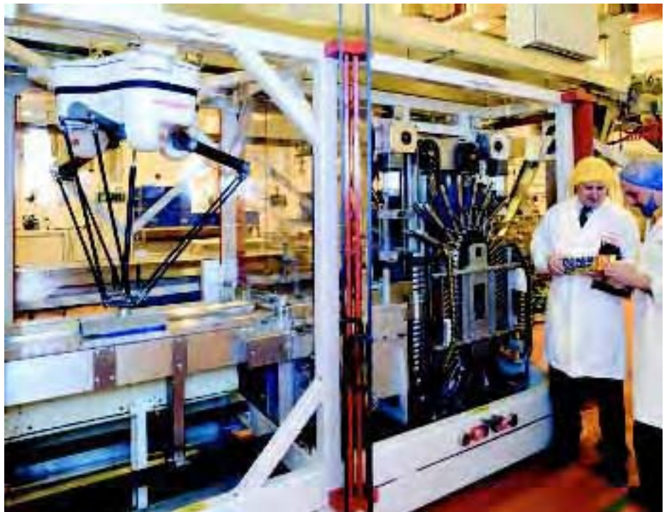
Creating 'bumper packs': Sewtec multipacker at Fox's uses two ABB FlexPicker robots for transfer duties
