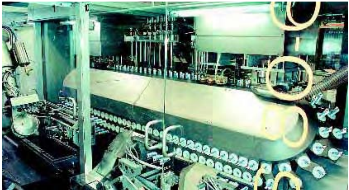
Twin track: IWKA TFS 80-6 tube filler showing robot loading and unloading of the containers
