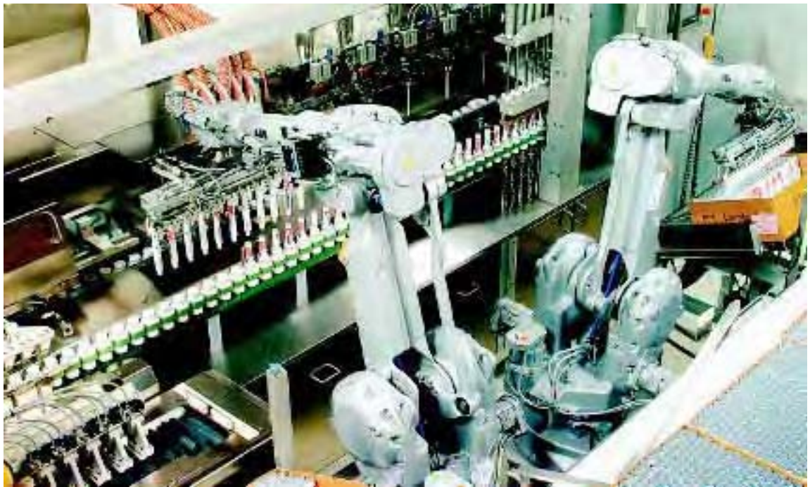
Top of range: Norden's high speed tube filling machine is the NM 5002S-HA capable of speeds up to 500 a minute
