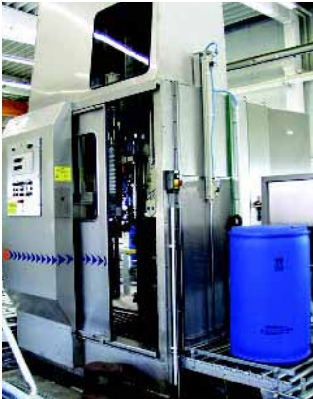
In-line: Feige automatic drum filler with enclosure
