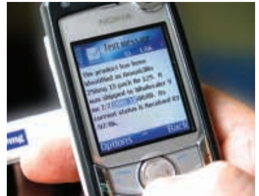
Checking authenticity: The bar code is scanned and sent to the database for checking. The user then receives the verdict
