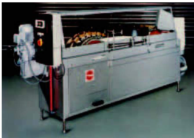
No sizeparts: Niko air cleaner has adjustable rubber belts to carry containers
