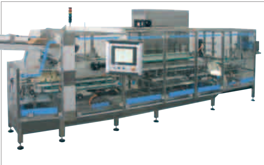
High speed sleeving: Cama machine produces 'upper bridge' style multipacks at speeds up to 250 a minute
