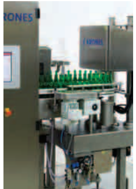
Empty bottle inspection: Krones' new K714 scans up to 18,000 containers an hour
