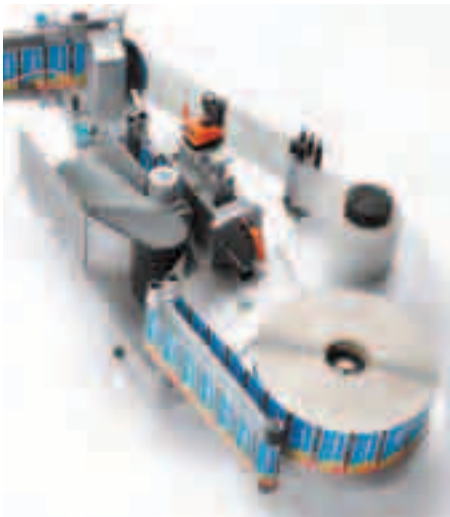
Changing to p-s: Herma 400 slimline applicators can be installed on existing wet-glue rotaries
