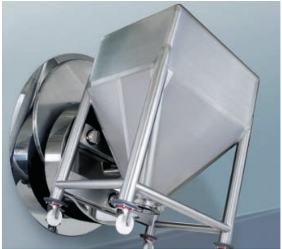
In-bin mixing: Above: IMA Vima Cyclops system. Below: Syspal Euro-bin Tumbler
