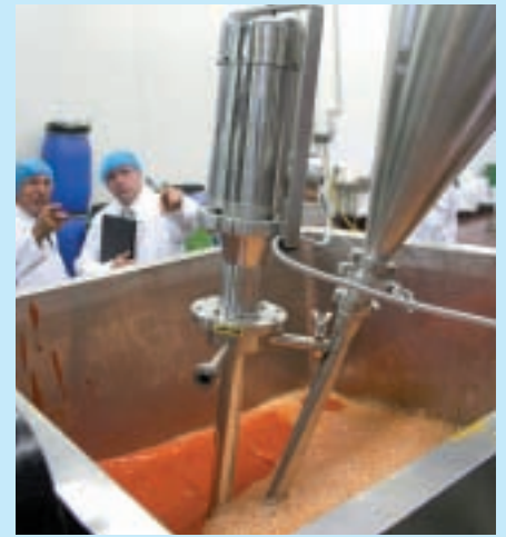
Stainless motor: Ytron-Y ByPass all-stainless high shear mixer at David Berryman
