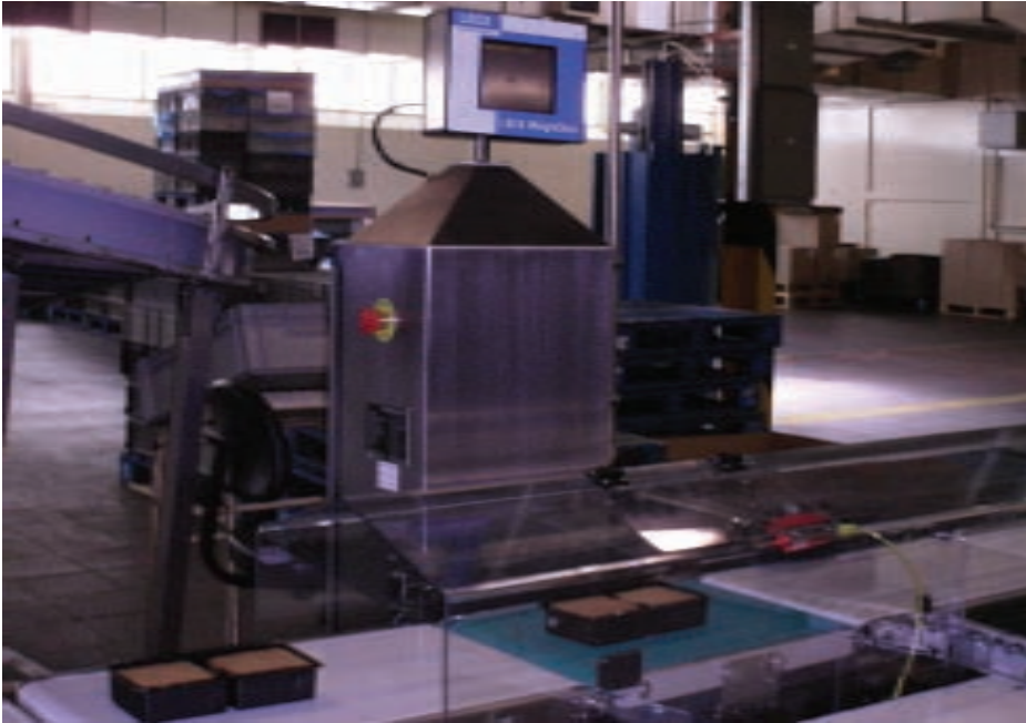
Monitoring biscuits: United Biscuits has installed a CK1500 checkweigher from Lock Inspection
