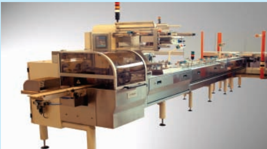
OPM-Jointech range: The J-200, capable of 300 packs a minute is one of the models now available in the UK
