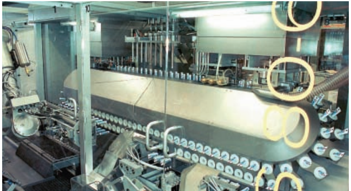
Twin track: Oystar-IWK TFS 80-6 tube filler showing robot loading and unloading of the containers
