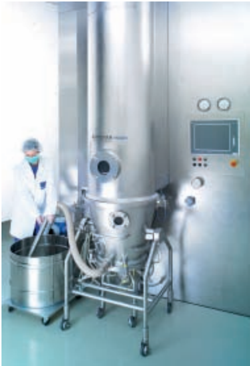
The new Ultraclean System from OYSTAR Hüttlin and the Pilotlab fluid bed system which has the ability to open the metal filter during CIP cleaning
