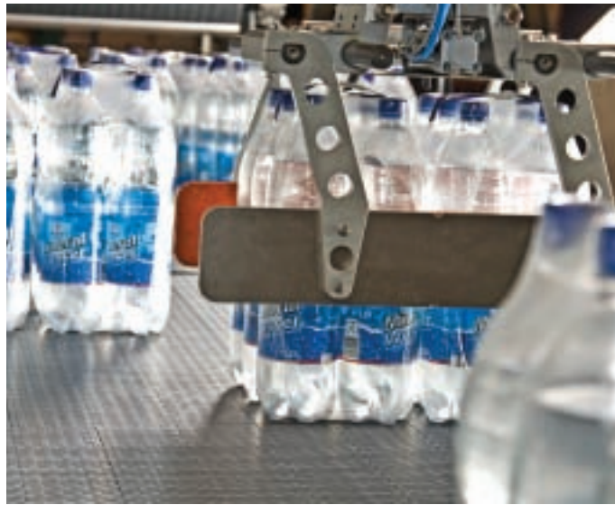
The Robobox pack grouping station from Krones
