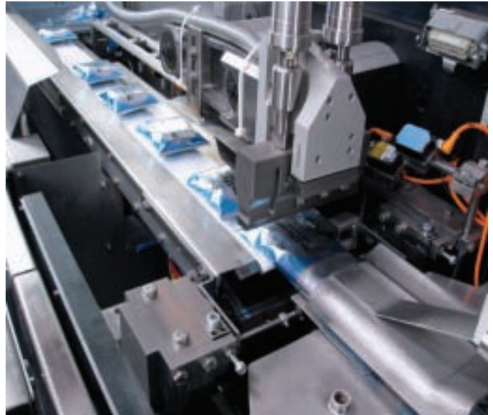
Ultrasound Sealing Technology for horizontal flow wraps - a packaging solution for temperature, steam and oxygen sensitive products
