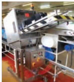
Three tray denesters have been installed at Jacob's
