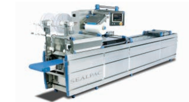
ThermoSkin packs can be produced on all Sealpac standard thermoformers such as this RE25 model
