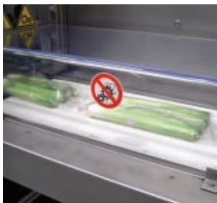
The LVA system handles random length products such as leeks and celery
