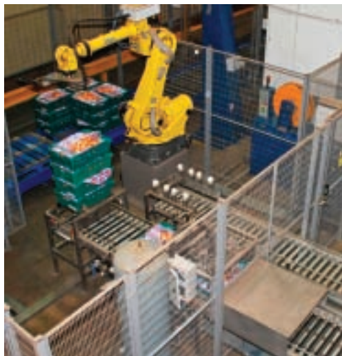
End of line packing system for loose onions at G's
