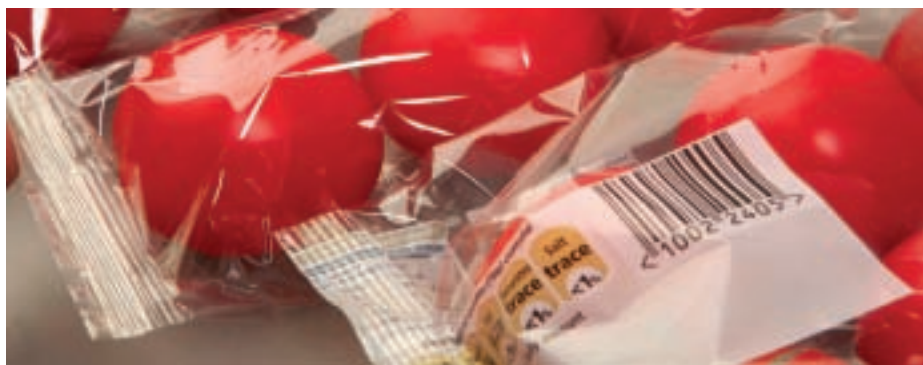
The PFM Falcon flow wrapper can pack tomatoes without a base tray, thus saving materials
