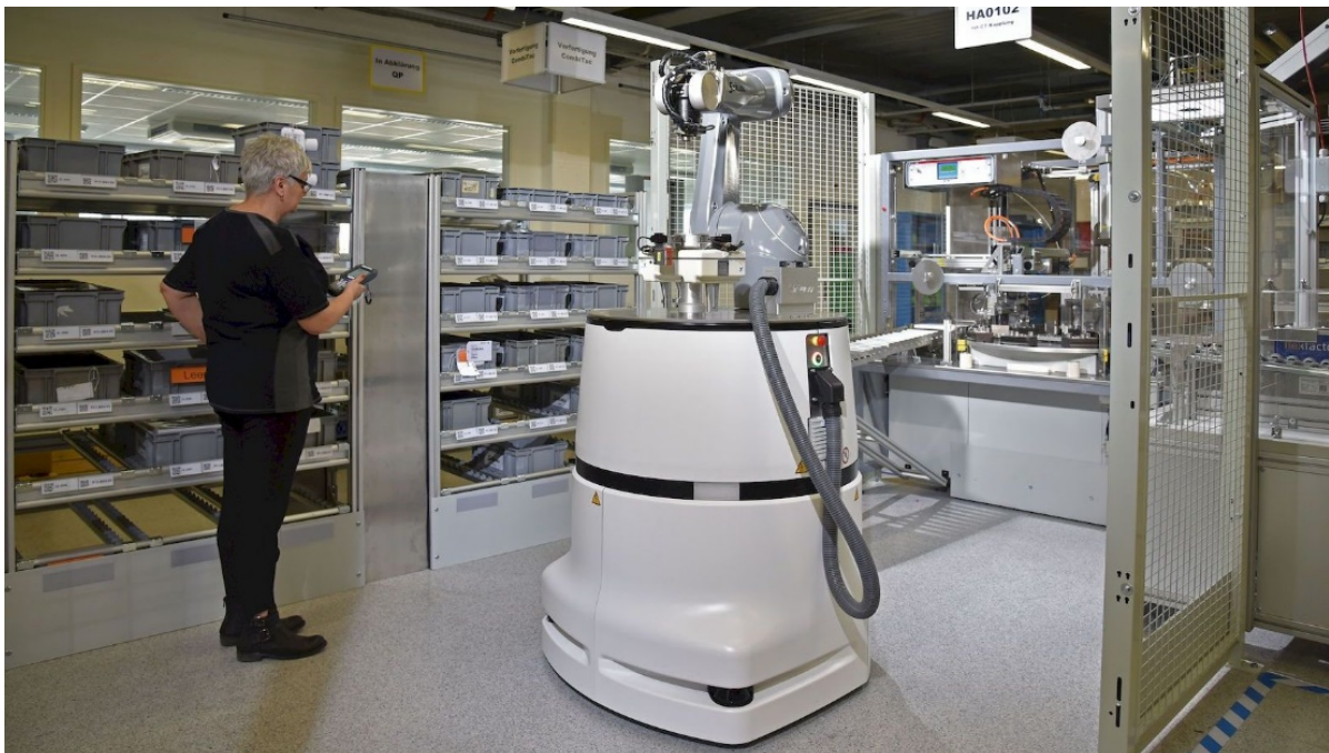
Figure 2: Mobile robots feed machine workstations. Image credit Stäubli
